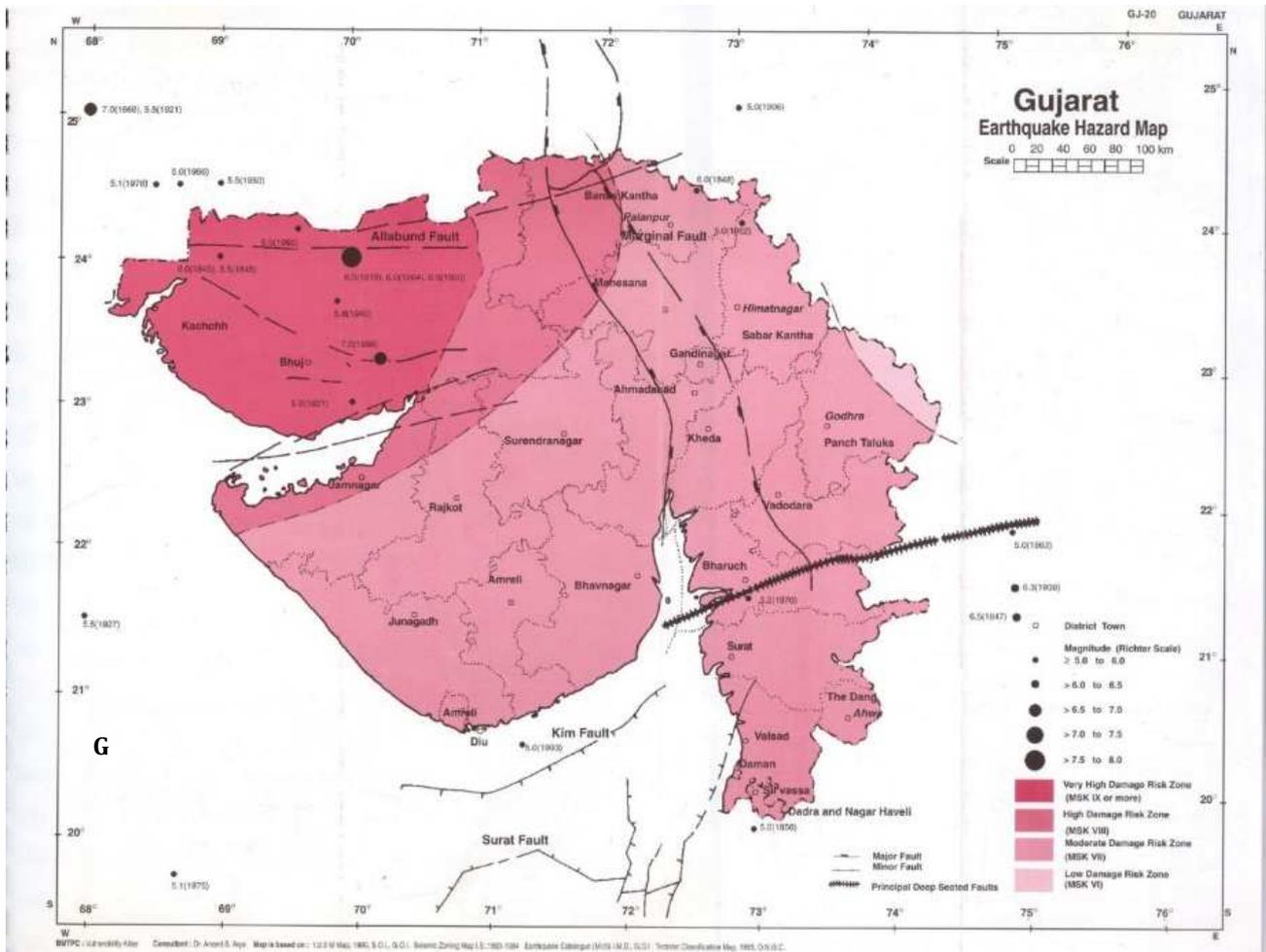
**Figure 2. Zoomed Gujarat portion of the Seismic Zoning Map of India which also corresponds to realistic Intensity distribution during Bhuj 2001 earthquake . Locations of some past earthquakes are shown.**
