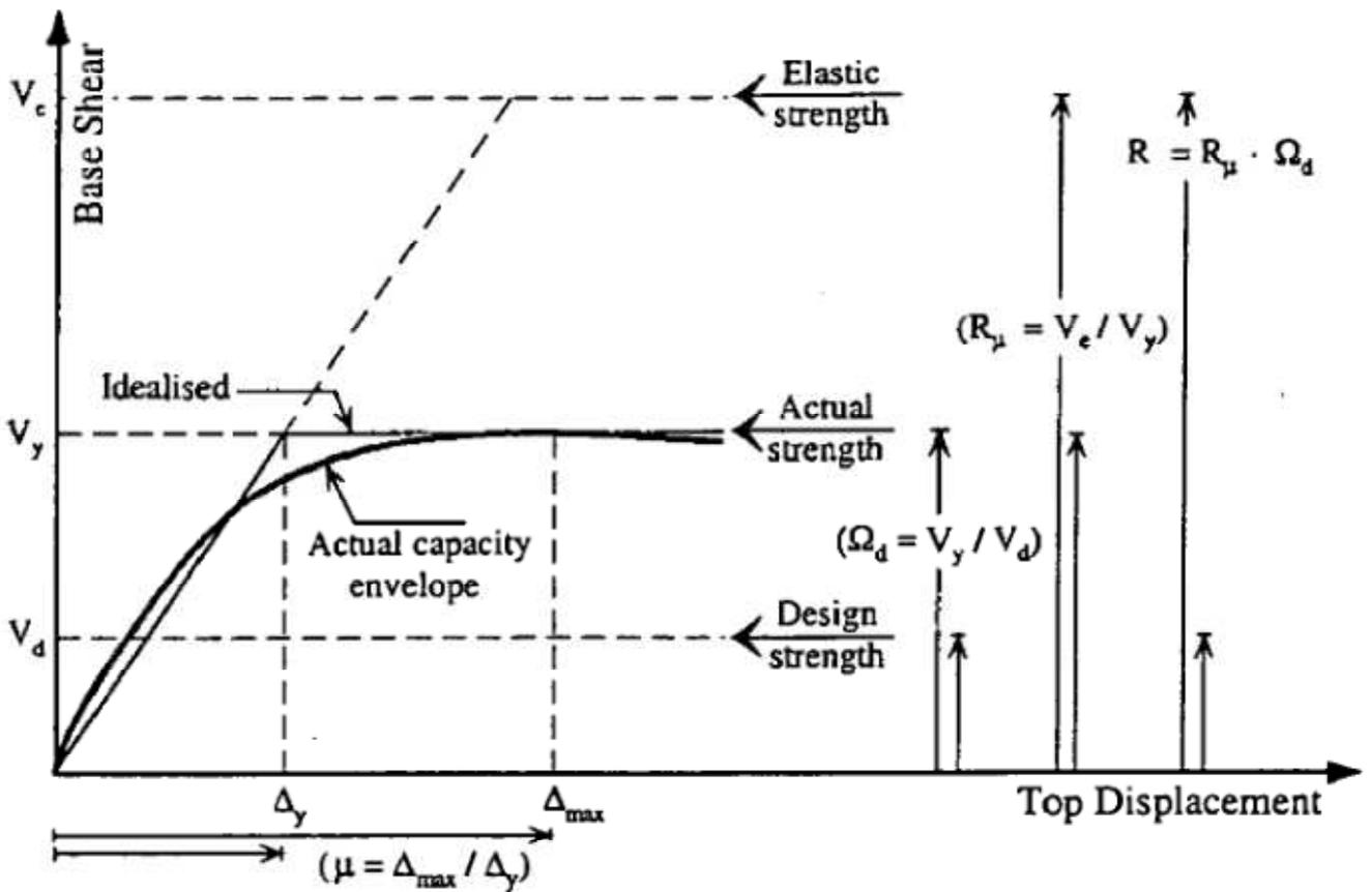
**Figure C3.** Relationships between the Force Reduction Factor  $R$  and Structural over Strength Factor  $\Omega_d$  and the Ductility Reduction Factor  $R_{\mu}$  (modified after Mwafy and Elnashai, 2002)
